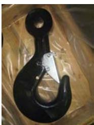
Our **Shackle Eye Hook** (LEFT) features an eye of cylindrical section for a close fit onto the shackle pin, limiting motion relative to the shackle, or other pin and evenly distributing the load. Shackle eye hooks are similar to DIN 15401 shank hooks and are forged from the class V alloy steel material noted above. Design factor is 5:1. Shackle Eye Hooks include a locking safety latch and can also be adapted for ROV (remote-operated vehicle) use.
