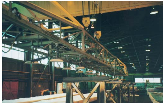
Bridge truss type unit used by a major aluminum producer to load finished aircraft wing skins into shipping container.
