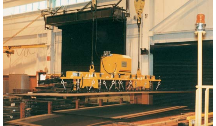
Custom 33" square pad vacuum lifter used on a shear line.
