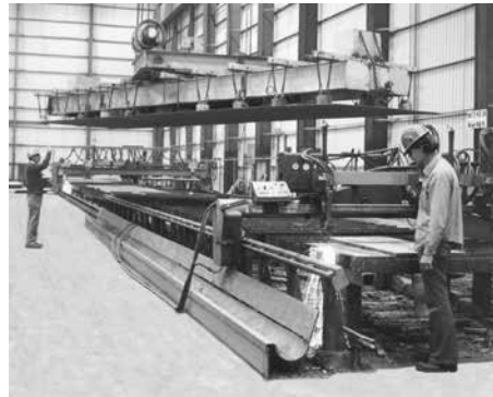
Multiple Selecto Magnets on a lift beam efficiently handle large steel sheets. In this installation, plates up to 10' x 50' x 4" (3 m x 15 m x 102 mm) are sorted and transported. The operator has precise remote control of every magnet so those not in use can be turned off, and single sheets can be placed when desired from multiple-sheet lifts.
