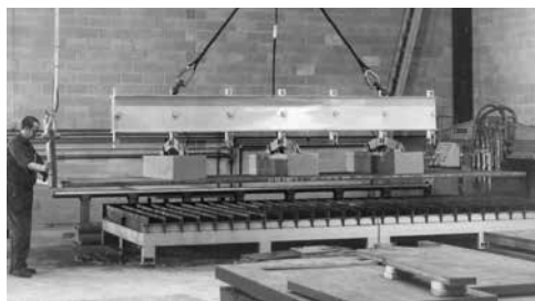
Heavy-Duty Rectangular Magnets provide maximum efficiency in multiple-plate handling applications like this.
