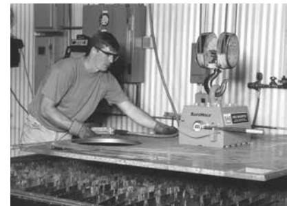
A Safehold® Permanent Magnet makes many lifts practical even with only minimum contact.
