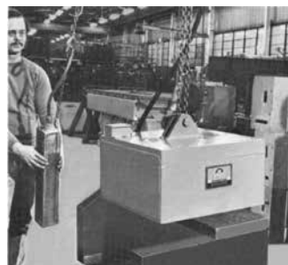
The Eriez Heavy-Duty Rectangular Magnet is effective in single or multiple-magnet applications for handling heavy fabrications or for lifting several thicknesses of sheet or plate at one time.
