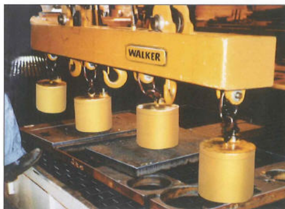
4 Walker Circular Magnets load and unload cut parts and skeletons from burning tables
