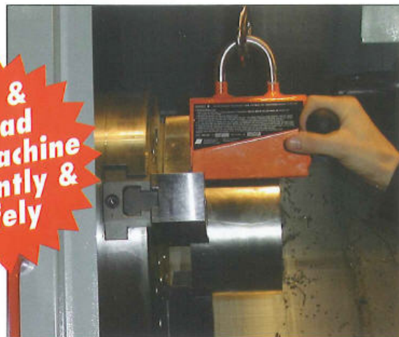
Small, but effective, 22 lb. Walker High-Powered NEO-250 magnets can lift up to 275 lb. Solid Round Bars
