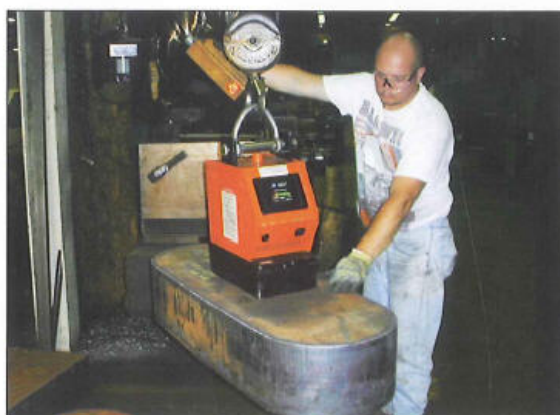
Infra-Red Remote Control Walker Self-Contained Battery Lift Magnets can lift steel up to 11,000 lbs.
