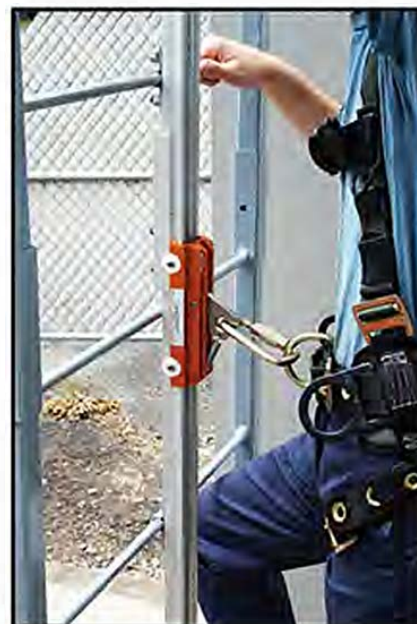
Ladder / Rigid Rail Climbing System in use
