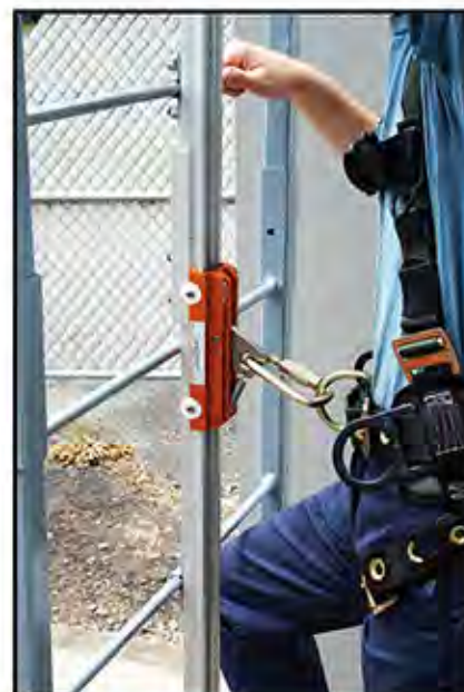
Ladder / Rigid Rail Climbing System in use
