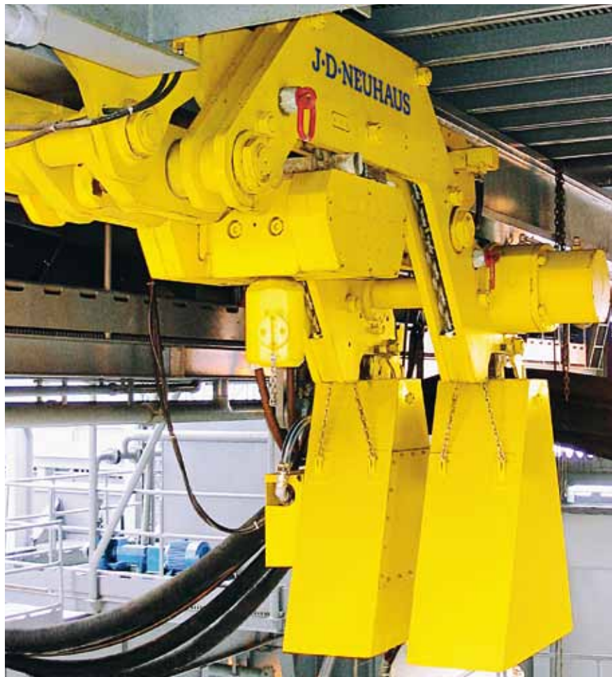
Ultra Low Headroom BOP Handling System BHU 200
