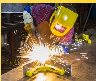
Each magnet holds on two sides.
