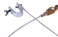
Part# 272031 All Purpose Bond Wire: For bonding drums to each other, to containers being filled, and to racks. Three-foot-long heavy duty wire rope with "C" clamp on one end and alligator clip on the other. Minimum order Qty. 5.
