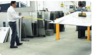
Stay safe. This extremely powerful On/Off Permanent Rare Earth magnet lets you guide loads into position without being in close proximity. Attach On/Off permanent magnet to a corner or along the side of your load.
